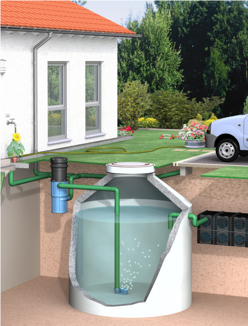
Example: Upstream to a rainwater harvesting tank.
